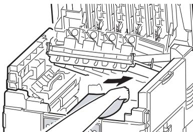
4. If paper is jammed in the fuser unit, push the lock lever (3) in the direction shown to release the unit.
