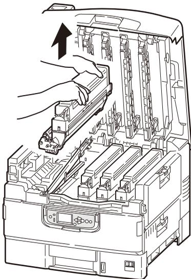
3. Turn the blue lock lever (2) of the toner cartridge to the direction of the arrow until it stops to release the lock.
