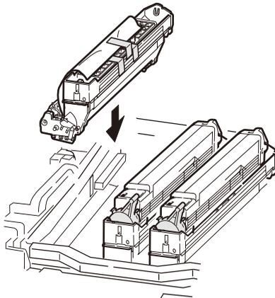
5. Pinch the both ends of the protective sheet with the thumb and index finger while holding down the image drum cartridge with other fingers, and pull out the protective sheet to the direction of the arrow.
