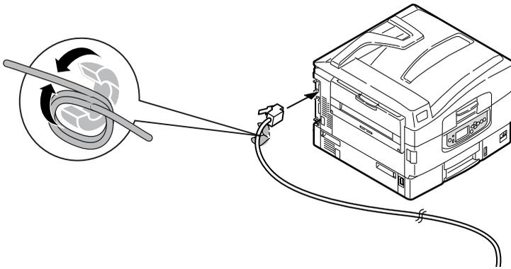
3. Connect an Ethernet cable between the printer and an Ethernet hub.
