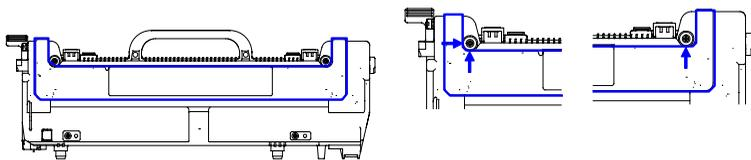
5. Carefully replace the fuser unit into the printer and turn the lock lever (5) in the direction of the arrow to lock the fuser unit.
