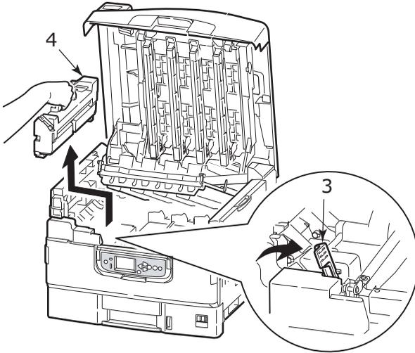
3. Remove the fuser cover sheet to which toner sticks from the fuser unit.
