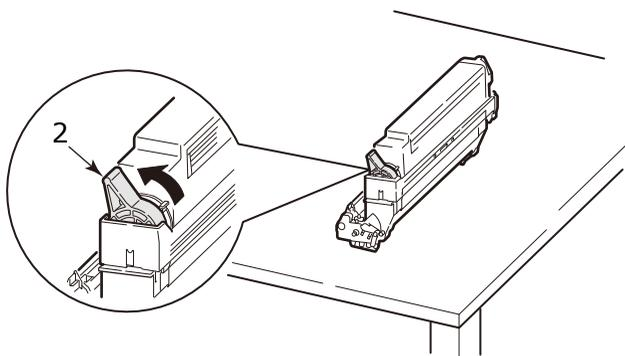
4. Lift up the toner cartridge carefully, and place it on the flat surface.
