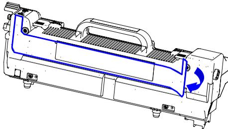
4. Remove the liner of the double-sided tape on the new fuser cover sheet, and attach the sheet to the fuser unit firmly.
