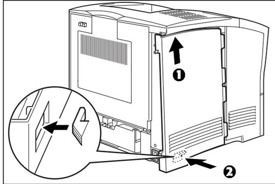
2. Slide the side cover towards the front of the printer to install it.
