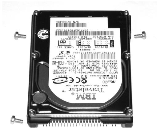
3. Use the three screws (1) provided to secure the bracket to the Hard Disk. Be sure to tighten the screws securely.
