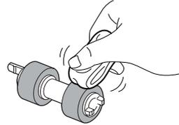
4. Turn the short tab of the feed roll to the right and slowly push it onto the shaft of the paper tray.
