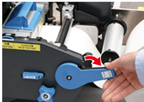
**18** After loading the paper, rotate the Roll Paper Guide Adjustment Knob counterclockwise and align the Roll Paper Guide to the width of the paper.
