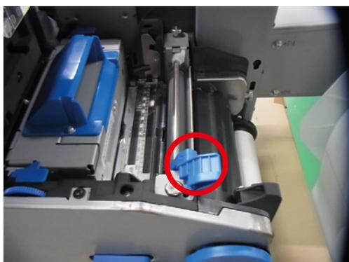
**12** Press the Tension Bar Open Lever upwards until it clicks.
