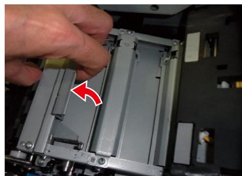
**16** While the paper guide release lever is lifted, slide the paper guide in the direction of the arrow to remove it.
