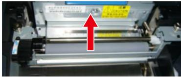
**21** As you rotate the gears with one hand, use Wiper moistened with cleaning fluid (anhydrous) to clean the top and bottom rollers on the F0 roller unit by wiping in just one direction.
