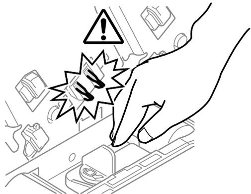
**9** Hold the belt unit handles (blue) on the left and right, and remove the belt unit at an angle.
