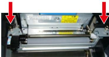
**23** Use Wiper moistened with cleaning fluid (anhydrous) to wipe, in one direction, the dirt off the sensor cover (upper).
