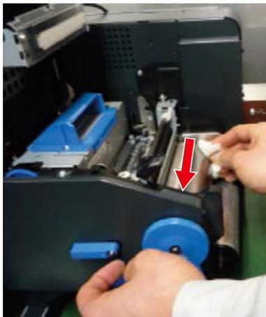
**15** Move the roll paper guide to confirm that there is no glue or paper scraps on it. If there are scraps of paper or glue from the labels on it, use Wiper moistened with cleaning fluid (anhydrous) to wipe it off.
