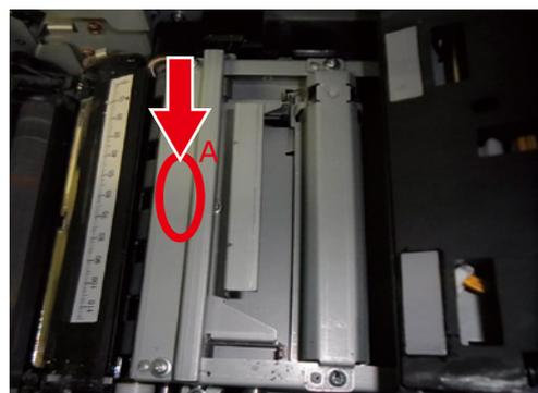
**34** Tilt the belt unit and align the arrow labels (red) on the belt unit and printer to position it, and then open the belt unit handles (blue) on the left and right.
