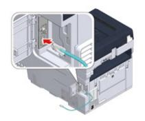
**5** Pass the LAN cable under the tab, and then close the interface cover.
