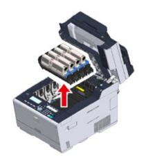
**5** Cover the removed image drums with paper so that the image drums are not exposed to light.
