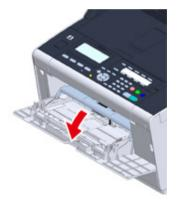
Pull out the paper support by holding the center part of it.
