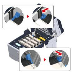
8 Hold the fuser unit handle and lift the fuser unit out of the machine.
