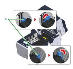
**16** Replace the four image drums into the machine
