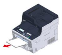
3 Hold the handle (B) and open the scanner unit (a) completely.
