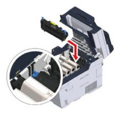
11 Push the levers on the fuser unit to lock.
