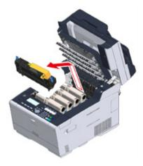
**9** Push the blue lever on the fuser unit and remove the orange safety stopper and film.
