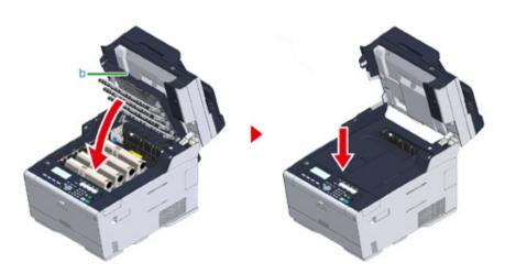
**15** Hold the handle (B) to close the scanner unit (a).
