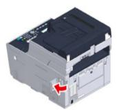
**1** Insert one end of the LAN cable into the network interface connector.
