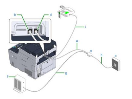
Plug one end of the included telephone cable (a) into the LINE connector (b) of the machine and the other end into a phone line splitter (e).
