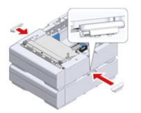
3 Slowly stack the machine on the additional tray unit aligning their back sides and right sides.
