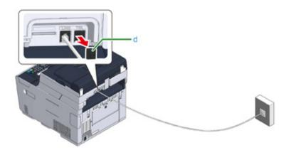
**3** Plug the telephone cable (f) that is connected to the external telephone into the TEL connector (e) of the machine.
