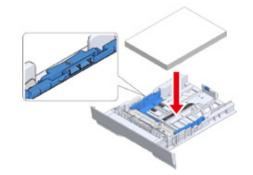
Secure the loaded paper with the paper guide.
