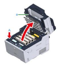
6 Pinch the tip of blue lever of the toner cartridge and turn forward until the tip aligns on the lug of the cartridge.
