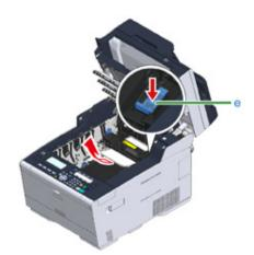
**8** Tilt the lock levers (f) on the both sides of the fuser unit toward you.
