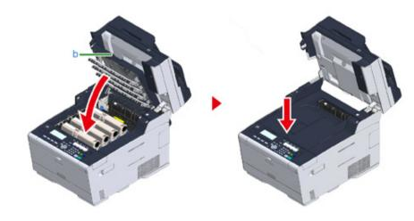
**16** Hold the handle (B) to close the scanner unit (a).
