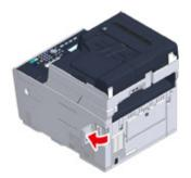
Insert one end of the USB cable into the USB interface connector on the machine.
