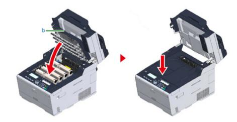
**18** Hold the handle (B) to close the scanner unit (c).
