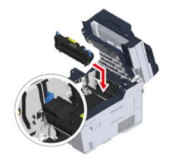
**15** Tilt the lock levers (f) on the both sides of the fuser unit.
