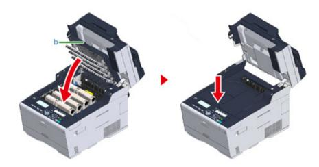
5 Hold the handle (B) to close the scanner unit (a).
