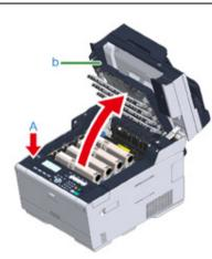
**4** Remove the four image drums from the machine and place the image drums on a flat surface.
