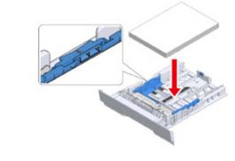
6 Secure the loaded paper with the paper guide.
