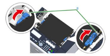
**14** Hold the fuser unit handle and place the fuser unit into the machine.
