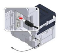
5 Pass the USB cable under the tab, and then close the interface cover.
