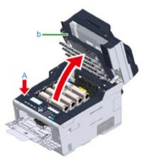
**5** Remove the four image drums from the machine and place the image drums on a flat surface.
