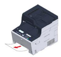
If jammed paper cannot be found, check the positions of the paper guides and paper stopper in the cassette and ensure that paper is correctly loaded.
