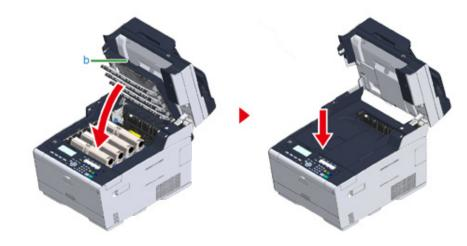
**1** Hold the handle (B) to close the scanner unit (a).
