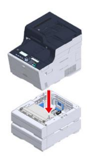
**/** Screw the machine and additional tray unit with the lock pieces.
