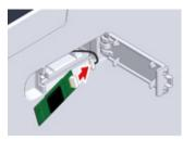
Install the wireless LAN module to the machine.
