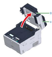
**3** Press the button (A) and open the output tray (b) completely.
