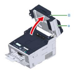
Press the button (A) and open the output tray (b) completely.
