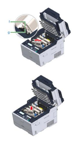
11 Hold the cartridge, pinch the tip of blue lever (c) of the toner cartridge, and turn forward until the tip aligns on the lug of the cartridge.
