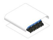
7 Open the transparent cover (c) inside the machine, remove the jammed paper slowly by pulling the edge of paper.
