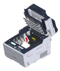
7 If paper jams in the fuser unit, press the jam release lever (e) on the fuser unit and slowly pull the jammed paper toward you.
