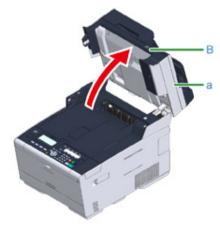
**5** Press the button (A) and open the output tray (b) completely.
