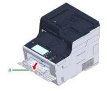
2 Slightly lifting the MP tray (a), press the right arm (b) inward, then unlock the tab (c).
