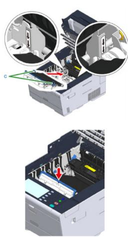
**9** Turn the lock levers (c) on the both sides of the belt unit backward.
