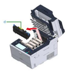
6 Push the blue lever on the new fuser unit and remove the safety stopper.
