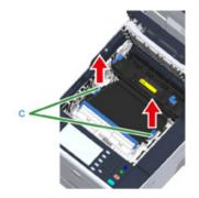
8 Hold the lock levers (c) of a new belt unit and place the belt unit into the machine.
