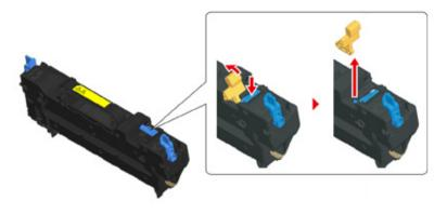
7 Hold the handle of a new fuser unit, align the fuser unit to the grooves behind the toner cartridges, place the fuser unit into the machine.
