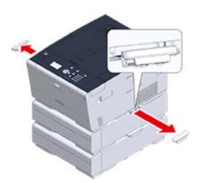
Lift up the machine to remove the additional tray unit.
