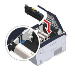
7 Tilt back the fuser unit lock levers (b) to lock.
