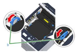
Remove the belt unit by holding the lock lever (b).
