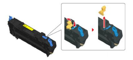
Hold the handle of a new fuser unit, align the fuser unit to the grooves behind the toner cartridges, place the fuser unit into the machine.
