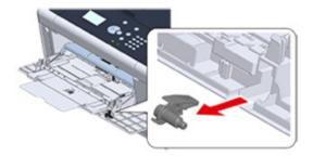
2 Remove the fuser unit from the machine. For details, see "Replacing the Fuser Unit".
