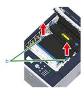
Hold the lock levers (b) of a new belt unit and place the belt unit into the machine.
