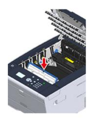
? Turn the lock levers (b) on the both sides of the belt unit backward.
