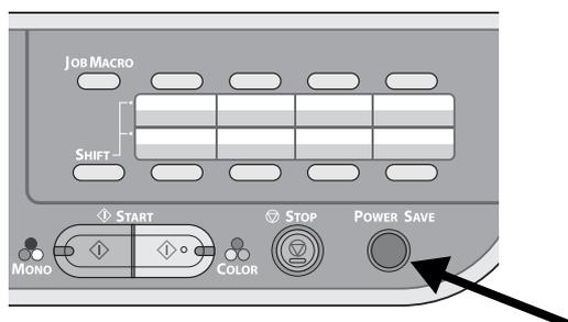
When your machine is not used for 30 minutes (the factory default), it automatically enters a power save mode to reduce the power consumption.
