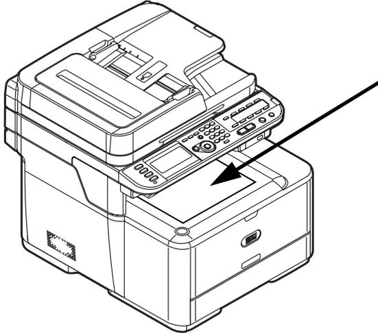
The top exit (facedown stacker) is the default. It is enabled when the rear exit is closed.
