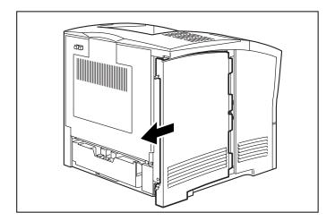
5. Turning thumbscrews counter-clockwise, remove the blank metal plate covering one of the available network ports on the controller bracket.
