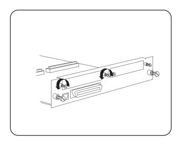
6. While aligning the front bracket of the serial interface assembly to the two respective thumbscrews on the controller assembly bracket, firmly seat the 80-pin male connector on the underside of the interface to the 80-pin female connector on the controller assembly.
