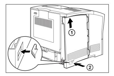
9. Slide the side cover towards the front of the printer to install it.
