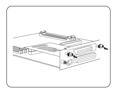
**8.** Insert the top part of the left side cover into the printer. Ensure the locking tab aligns with the hole in the printer's side.
