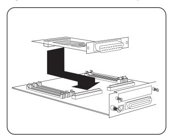
7. Secure the serial interface assembly to the controller bracket by tightening the two smaller thumb-screws in a clockwise direction.
