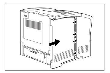
10. Tighten both thiumbscrews in a clockwise direction.
