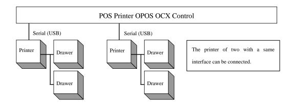
The POS Printer OPOS OCX control can use up to 255 of LAN simultaneously.
