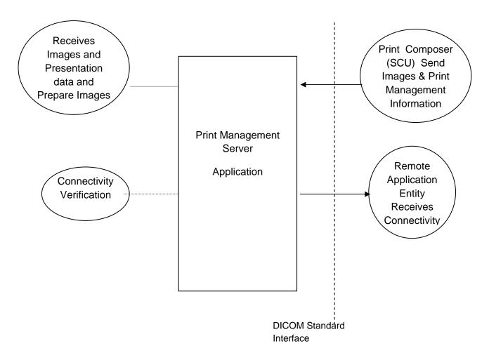
The Print Server is receiving the Images with the Presentation information, it applies it on the images and creates a print-job within the print queue, containing one or more film pages composed from images selected by the client Print SCU. Furthermore, it also manages the Printer Status and Configuration.
