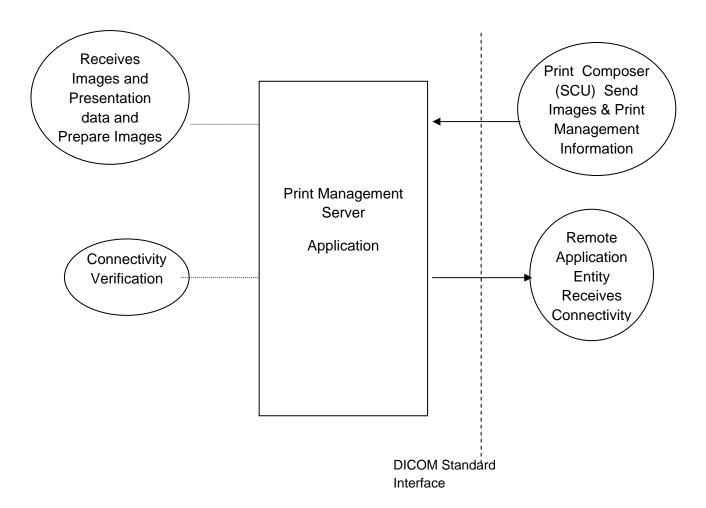
The Print Server is receiving the Images with the Presentation information, it applies it on the images and creates a print-job within the print queue, containing one or more film pages composed from images selected by the client Print SCU. Furthermore, it also manages the Printer Status and Configuration.
