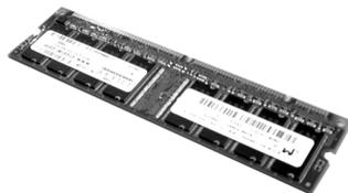
7. Insert the card in the slot and press firmly into place. Push the white tabs against the sides of the card to lock it in place.
