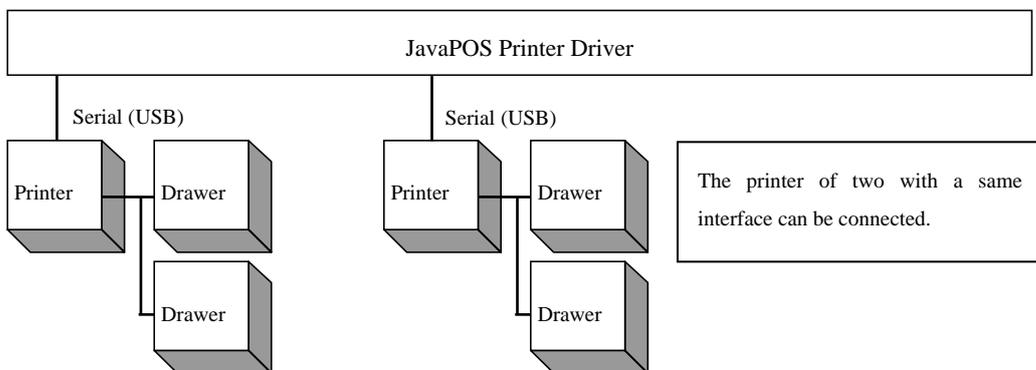
\* When you set two or more printers, connect printer one by one, and set it with the setup tool.
