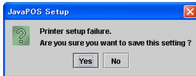
When the printer status is "error" and this setting program is executed, the setting is not reflected in the printer.
