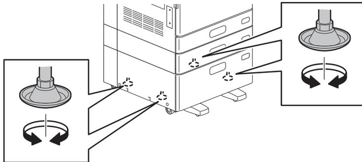
Before moving the equipment with the Desk installed, remove the front stabilizer. Be sure to reinstall it after the equipment has been moved.
