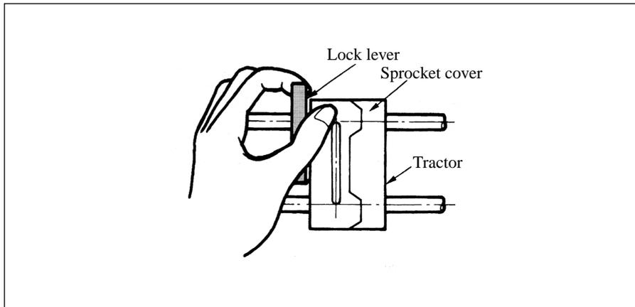
7. Pull the paper under the column indicator and up to the level of the tractor unit.
