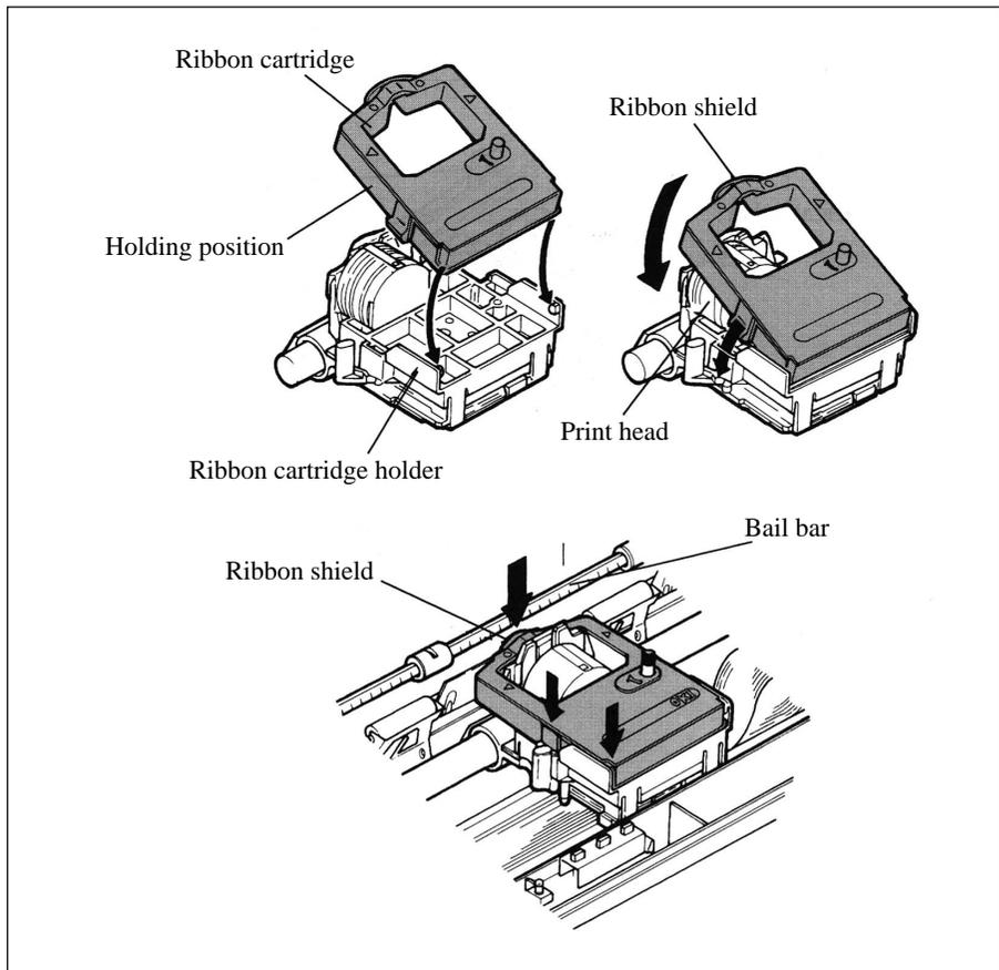
6. Press gently on the cartridge until you feel it snap into place. To remove the ribbon cartridge, make sure the print head is moved away from the edge of the platen, then grasp the cartridge on both sides of the print head and lift up.
