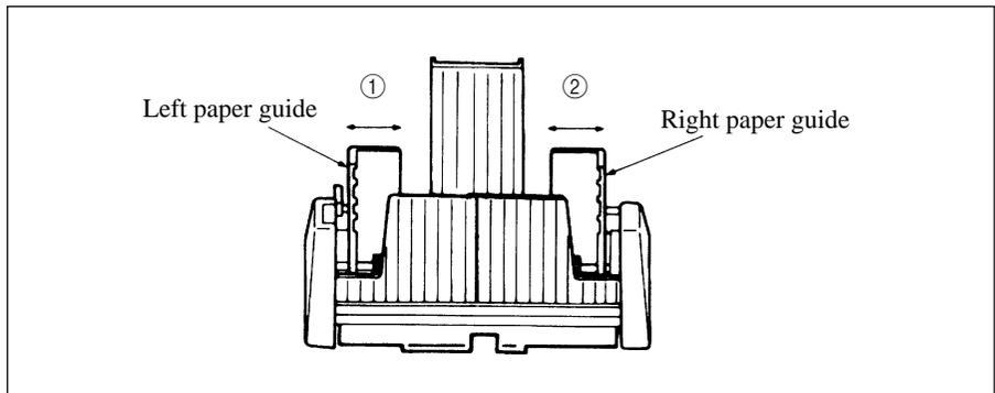
4. Flex the paper stack (not more than 170 sheets of 60g/m<sup>2</sup> (161b) paper). Square the stack again, turn it over, and repeat the bending. The paper stack should not exceed 16mm in total thickness.
