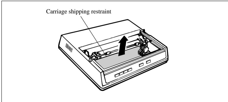
4. Gently slide the print head to the middle of the printer or to the lefthand side so that it is away from the rollers on the Bail bar.
