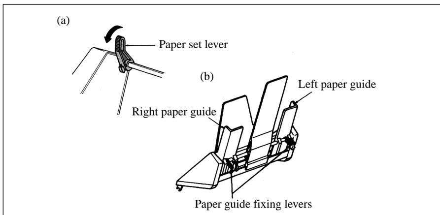
2. Release the paper guides by pushing the fixing levers downwards.
