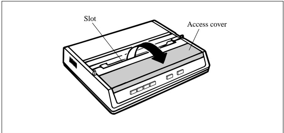
3. Remove the carriage shipping restraint that keeps the print head in place.
