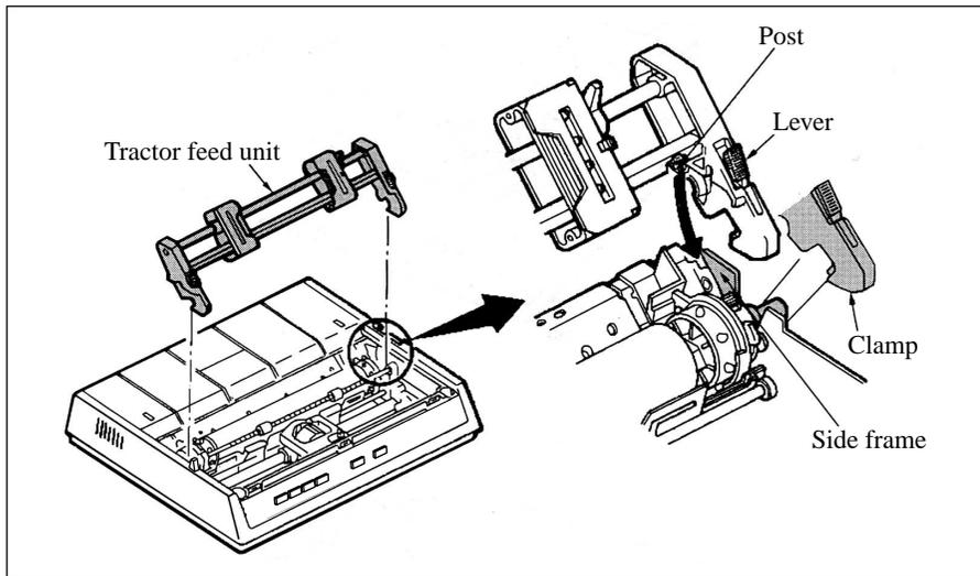
3. Pull the tractor unit forwards until it clamps on to the platen ends.
