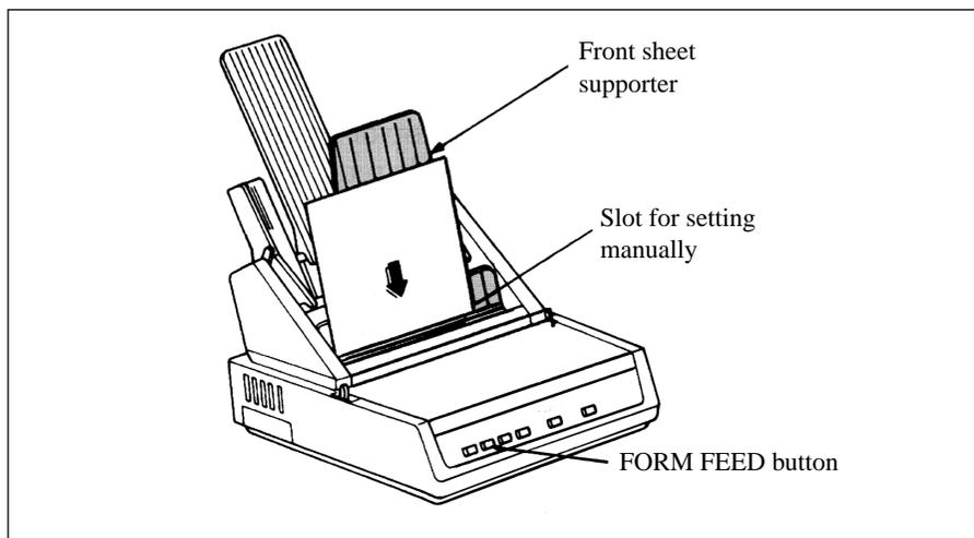
2. Use the FORM FEED button to feed the manually loaded paper.
