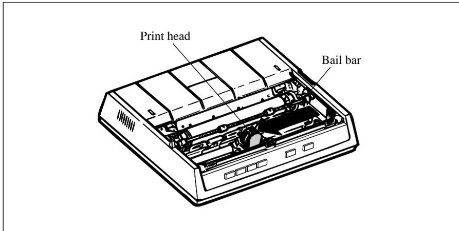
5. Place the black ribbon cartridge on the ribbon cartridge holder. The easiest method is to tilt the back of the cartridge so that it slides into the area of the plate that is nearest the front of the printer, then lower the top of the cartridge (where the plastic ribbon shield is located) over the print head. The tabs on both sides of the cartridge should align perfectly with the inserts on the print head plate.
