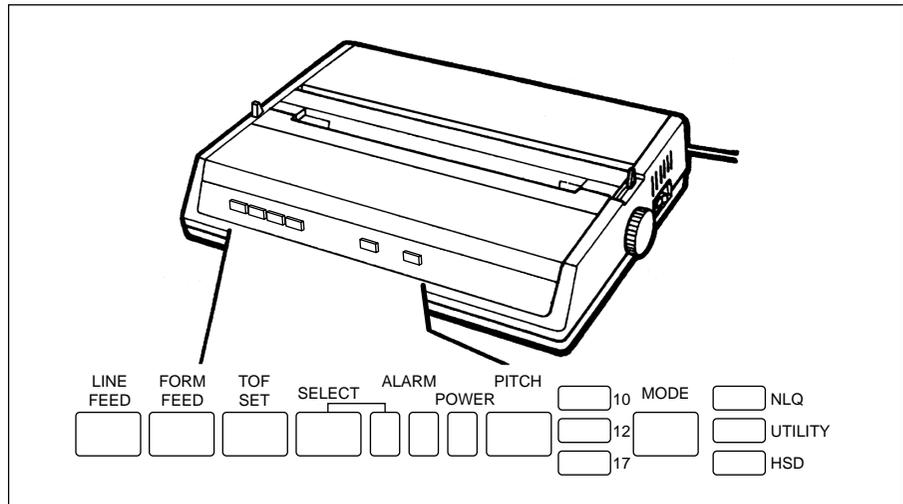
**POWER Indicator:** Indicates that the printer power is turned ON.
