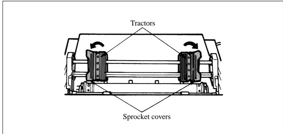
10. Place the sprocket holes in the paper over the sprockets on the tractor unit, making sure that the paper is flat.
