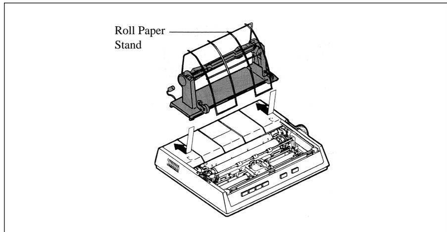
3. Plug the roll paper stand plug into the socket on the rear of the printer.
