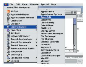
**2.** From the AppleTalk configuration page select [Connect via: Ethernet].
