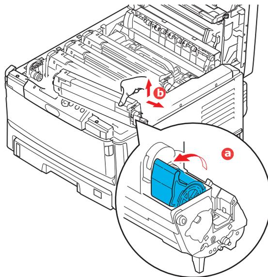
4. Lift the right-hand end of the cartridge and then draw the cartridge to the right to release the left-hand end as shown, and withdraw the toner cartridge (b).
