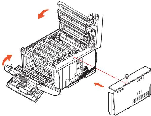
9. Close the front cover and the top cover, pressing down firmly at each side to latch it closed.
