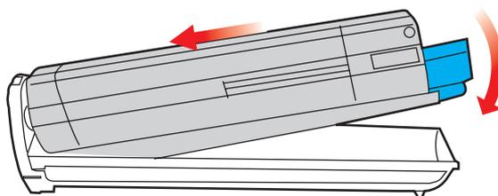
9. Push the coloured release lever away from you to lock the toner cartridge onto the new image drum unit and release toner into it.
