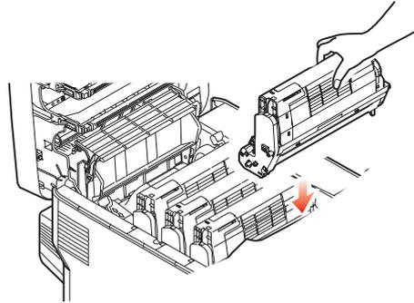
9. Lower the top cover but do not press down to latch it closed yet. This will protect the drums from excessive exposure to room lighting while you check the remaining areas for jammed sheets.
