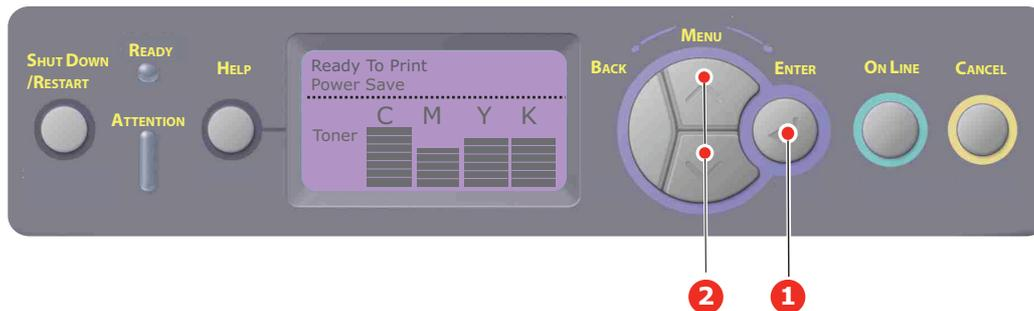
1. When the machine is idle use the UP or DOWN arrow buttons (2) to select the PRINT JOB menu, then press [ENTER] (1).
