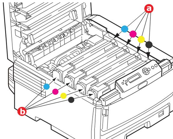
3. Lift each of the image drum units out of the printer and place them in a safe place away from direct sources of heat and light.
