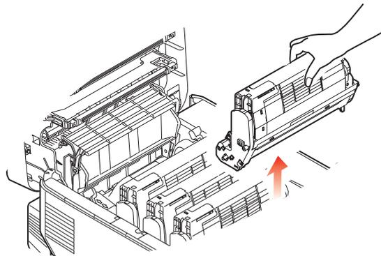
5. Put the assembly down gently onto a piece of paper to prevent toner from marking your furniture and to avoid damaging the green drum surface, and cover.
