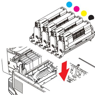
Holding the complete assembly by its top centre, lower it into place in the printer, locating the pegs at each end into their slots in the sides of the printer cavity.
