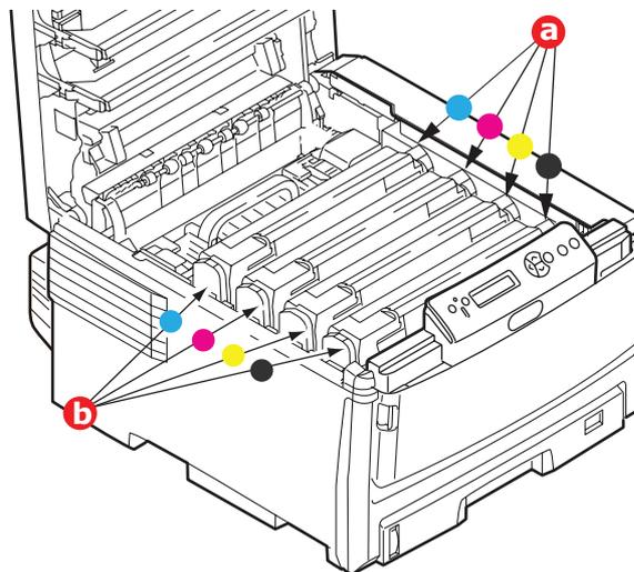
3. Holding it by its top centre, lift the image drum, complete with its toner cartridge, up and out of the printer.
