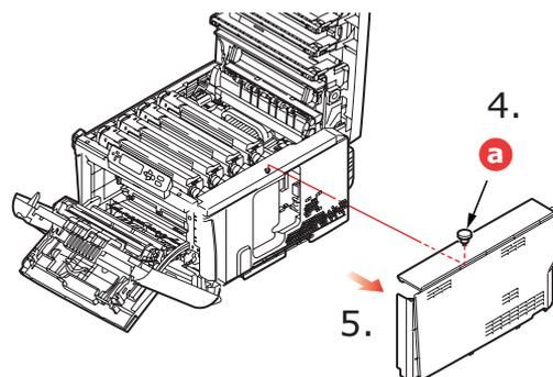
5. Lift the edge of the side cover slightly and pull the cover away from the printer at the top. Lift the cover slightly to detach it from the printer. Place it safely to one side.
