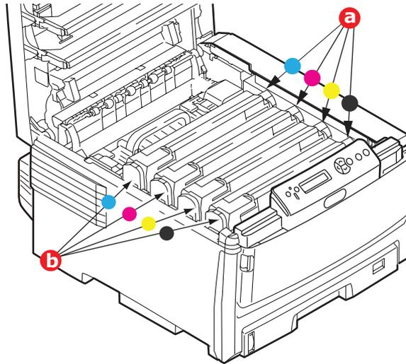
It will be necessary to remove the four image drums (b) to gain access to the paper path.
