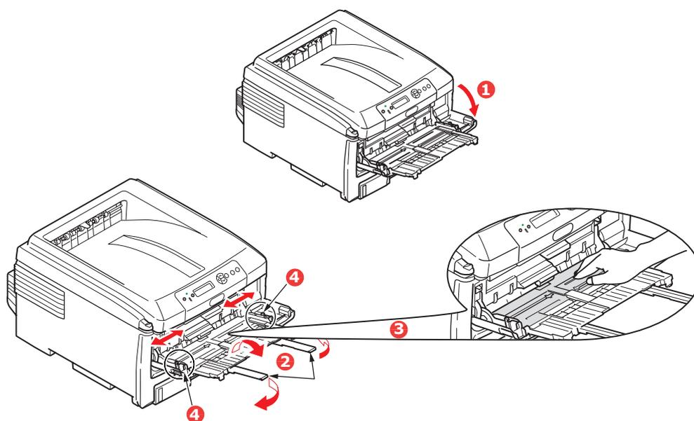
3. Press gently down on the paper platform (3) to ensure it is latched down.
