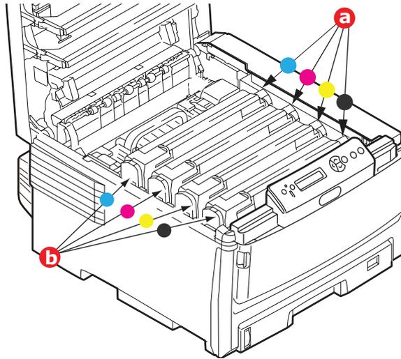
3. Pull the coloured toner release lever (a) on the cartridge to be replaced fully towards the front of the printer.
