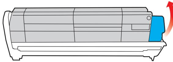
10. Holding the complete assembly by its top centre, lower it into place in the printer, locating the pegs at each end into their slots in the sides of the printer cavity.
