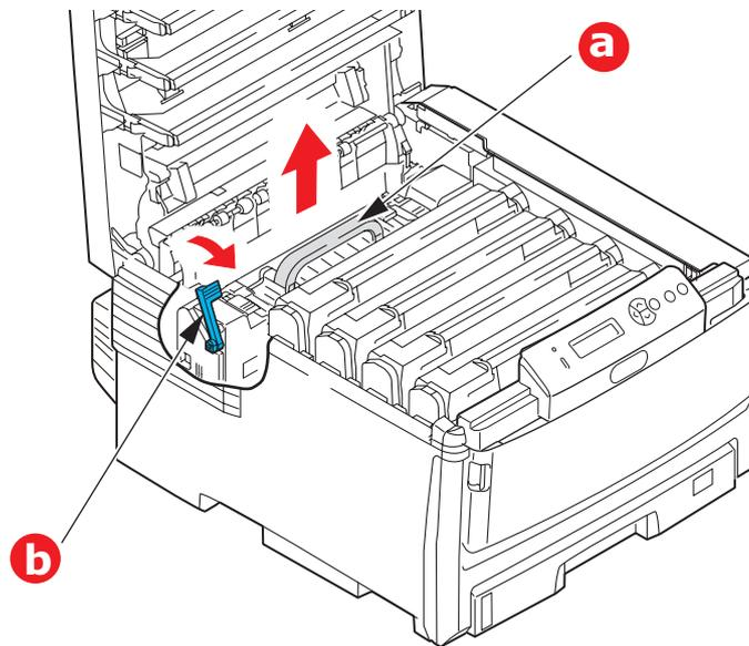
3. Pull the fuser retaining lever (b) towards the front of the printer so that it is fully upright.
