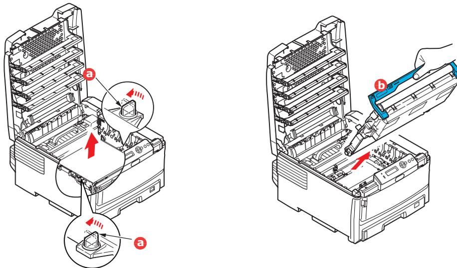
5. Turn the two fasteners 90° to the left. This will release the belt from the printer chassis.
