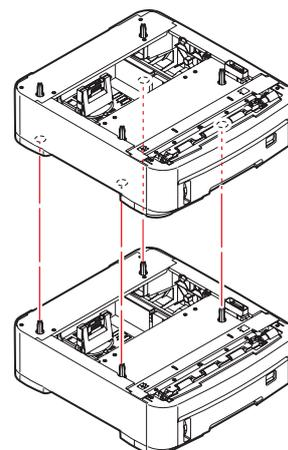
3. Observing safety rules for lifting and, using locating guides (a), place printer on top of the additional paper tray(s).
