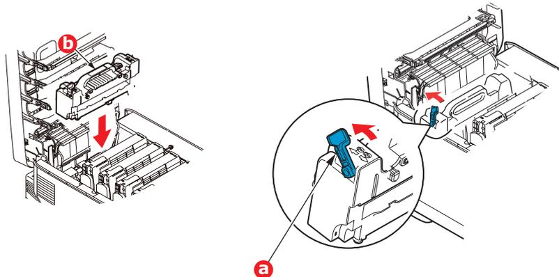
8. Starting with the cyan image drum unit nearest the fuser, replace the four image drums into the drum cavity, making sure to locate them in the correct order.
