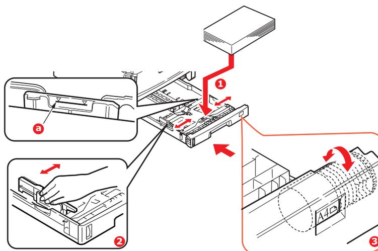
4. Adjust the rear stopper, paper guides (2) and cassette tray roller (3) to the size and orientation of paper being used. For A6 paper, remove and re-install in the A6 position.
