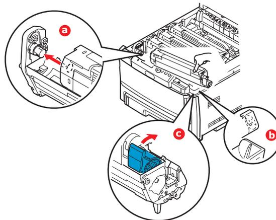
11. Pressing gently down on the cartridge to ensure that it is firmly seated, push the coloured lever (c) towards the rear of the printer. This will lock the cartridge into place and release toner into the image drum unit.
