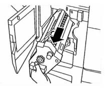
**5.** Turn the knob in the direction indicated to move the stapler to the front.
