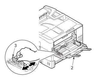
**3.** Adjust the paper guides (3) to the size of the paper being used.
