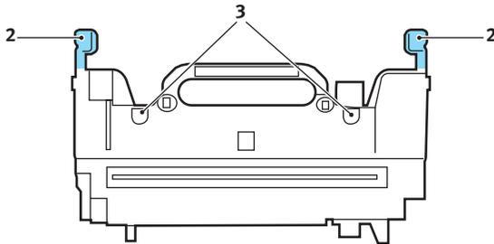
7. Lower the fuser into the printer, locating the two lugs (3) into their slots in the metal partition which separates the fuser area from the image drums.
