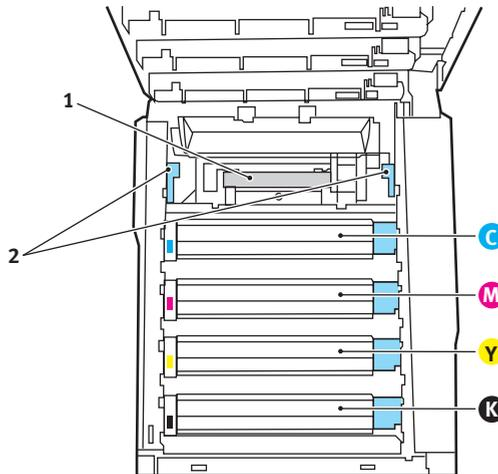
3. Pull the two fuser retaining levers (2) towards the front of the printer so that they are fully upright.
