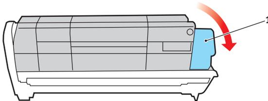
6. Lift the right-hand end of the cartridge and then draw the cartridge to the right to release the left-hand end as shown, and withdraw the toner cartridge out of the image drum cartridge. Place the cartridge on a piece of paper to avoid marking your furniture.
