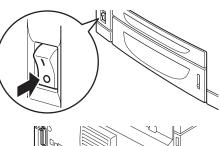
2. Connect the power cord to the power cord connector at the back of the printer. Connect the other end of the power cord to the power outlet.
