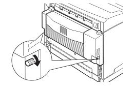
3. Tighten the screws at both ends of the bottom of the duplex unit.
