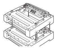
5. Insert the fasteners provided into the two locations inside the tray module and the two locations at the back of the tray module. Insert the fasteners securely.
