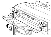
2. Push up the rear output tray lever as shown in the diagram (1) and pull out the extension tray (2).
