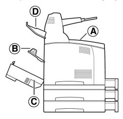
Cover A: When the optional offset catch tray is installed, fold the tray first before opening cover A. When a message to remove the drum-toner cartridge is displayed, refer to "Inside Cover A" on page 58.
