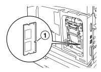
3. Release the hook on the top of the slot.
