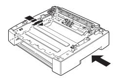
4. Align the front and back corners of the top and bottom tray modules, and slowly lower the top module so that the guide pins at the four corners of the bottom module fit into the holes at the base plate of the top module.
