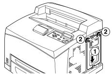
2. Align and insert the protrusions at the top of the right detachable cover into the notches of the printer (1). Fit the protrusions at the bottom of the cover into the printer (2) and slide the cover towards the front of the printer (3).
