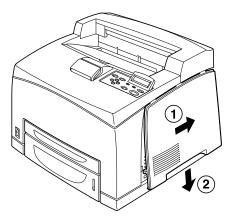
3. Remove the two screws on top of the metal cover (1), and pull the metal cover upwards (2).
