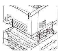
9. Insert the fasteners provided into the two locations inside and the two locations at the back of the printer. Insert the fasteners securely.
