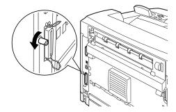
2. Slide the cover towards the back of the printer (1) to release the protrusions at the bottom and pull it downwards (2).
