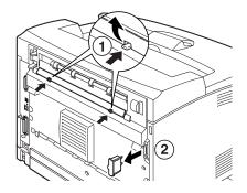
2. Insert the right and left tabs at the bottom of the duplex unit into the holes at the back of the printer, and then align the top part of the duplex unit with the printer.
