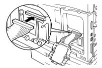
5. Hold the hard disk as shown in the diagram, and install it in the printer. Align the arrow on the hard disk with the arrow on the printer, and insert the bracket at the top of the disk into the install position.
