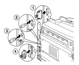
2. For Parallel, USB, or Serial cables, connect the other end of the cable to the interface connector of the computer.
