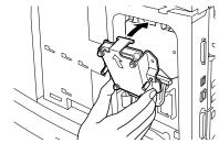
6. Tighten the screws on both sides of the hard disk.
