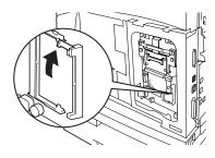
4. Gently insert the network software kit into the slot, and press firmly at the top corner of the card then at the bottom corner.
