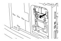
3. Locate the Compact Flash disk as shown in the diagram.
