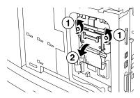
3. Remove the cable of the Compact Flash bracket from the connector on the printer.
