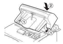
4. Secure the screws at both ends of the bottom of the offset catch tray.
