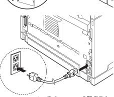
Press the power switch of the printer to the < > position. The power will be applied and the control panel will display that the printer is ready to print.
