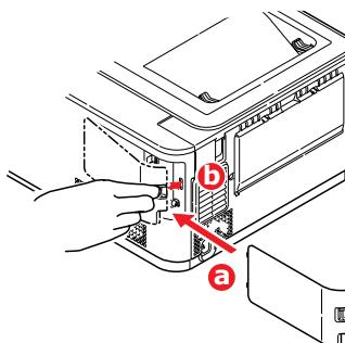
12. Reconnect the AC power cable and switch the printer on.
