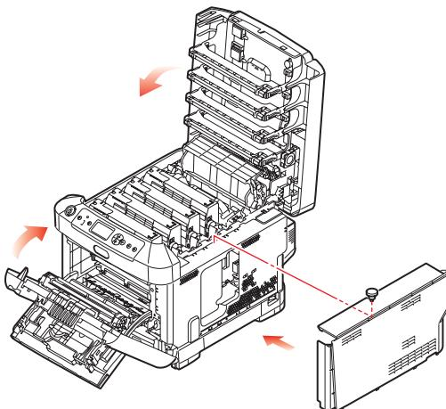
14. Close the front cover, and close the top cover, pressing down firmly at each side to latch it closed.
