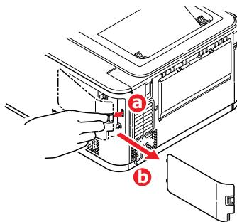
3. Turn locking screw (a) anti-clockwise and remove the inner access cover (b). Place it safely to one side.
