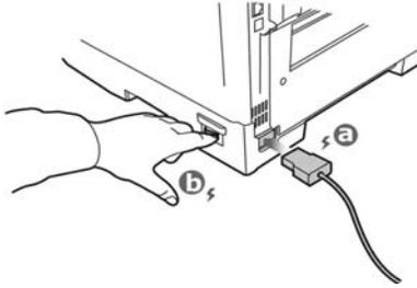
**WARNING!** Be sure to use only the power cable supplied with your printer! Use of a power cord not supplied with this printer, or an extension cord, could be a safety hazard.
