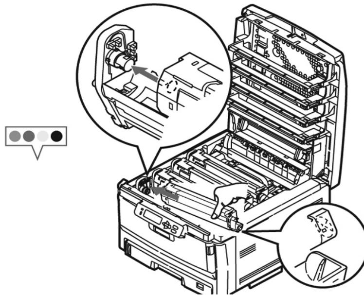
1. Place opening on left side of toner cartridge on image drum peg.
