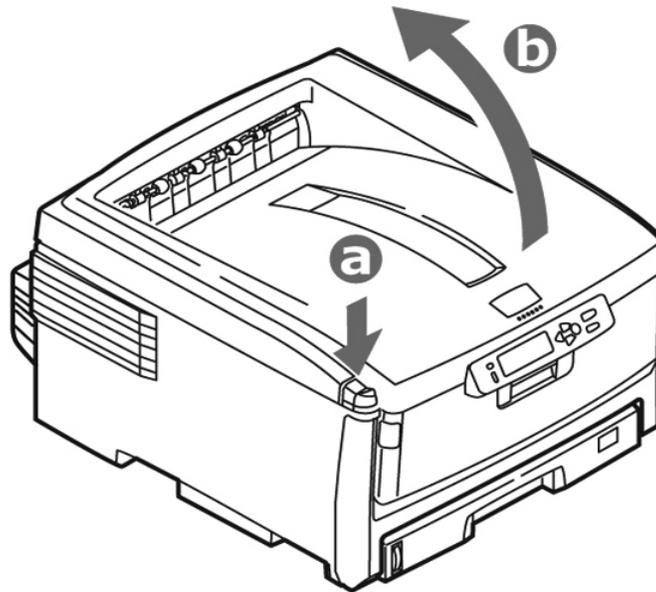
Press the release button (a) and lift the top cover (b).
