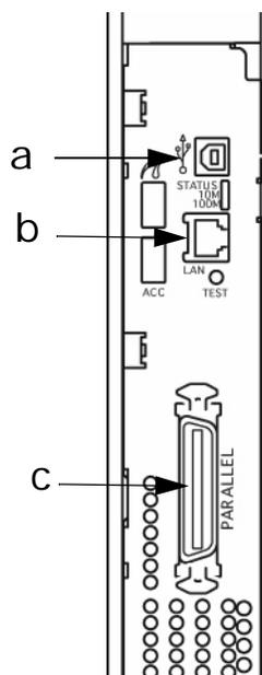
**Note:** Install printer software *BEFORE* connecting the USB (a) cable.
