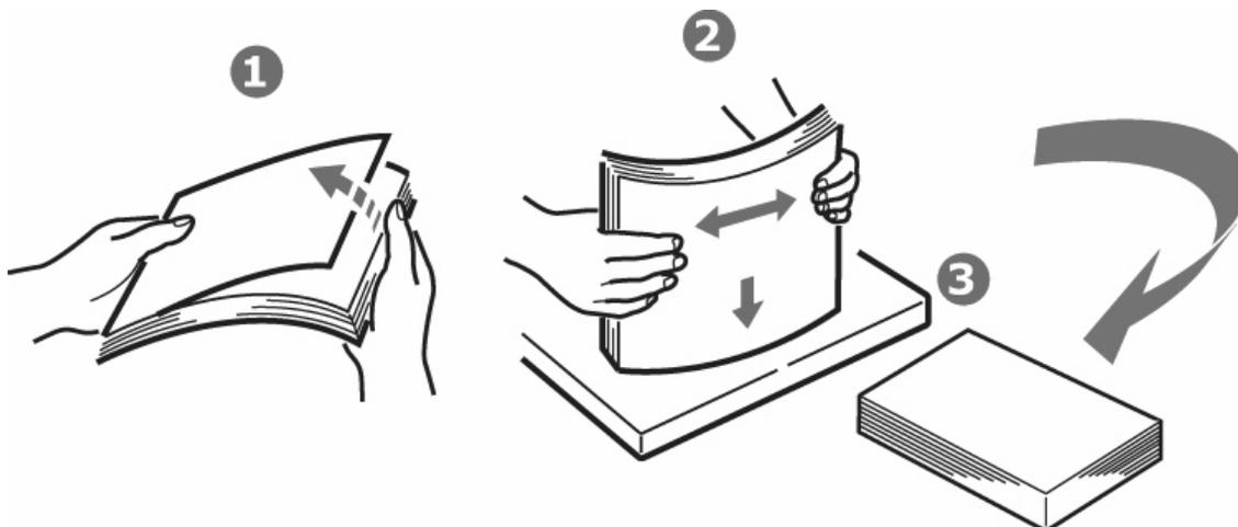
Fan the paper to be loaded at the edges (1) and in the middle (2) to ensure that all sheets are properly separated, then tap the edges of the stack on a flat surface to make it flush again (3).
