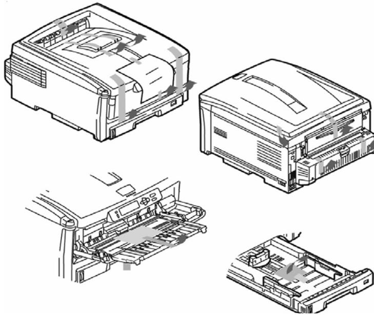
Remove the packing materials and shipping tape.
