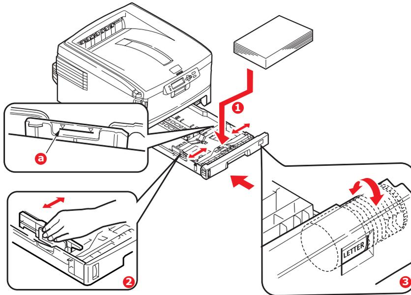
1. Load paper print side down, long edge feed (1) up to the mark (a). Letterhead: print side down, top edge towards the right side of the printer.
