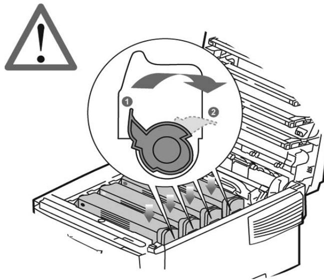
1. Push the lock lever toward the back of the printer *as far as it will go*.
