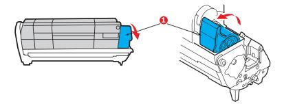
**6.** Lift the right-hand end of the toner cartridge (1) and then draw the cartridge to the right to release the left-hand end as shown (2), and withdraw the toner cartridge out of the image drum cartridge. Place the cartridge on a piece of paper to avoid marking your furniture.
