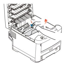
(c) To remove a sheet just entering the fuser (3), separate the trailing edge of the sheet from the belt, push the fuser pressure release lever (4) towards the front and down to release the fuser's grip on the sheet, and withdraw the
