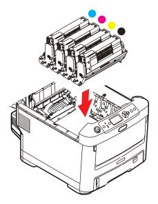
Holding the complete assembly by its top centre, lower it into place in the printer, locating the pegs at each end into their slots in the sides of the printer cavity.
