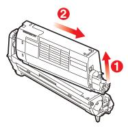
7. Take the new image drum cartridge out of its packaging and place it on the piece of paper where the old cartridge was placed. Keep it the same way round as the old unit. Pack the old cartridge inside the packaging material for disposal.
