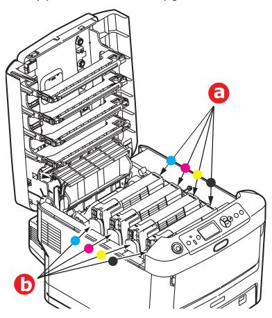
**3.** Holding it by its top centre, lift the image drum, complete with its toner cartridge, up and out of the printer.
