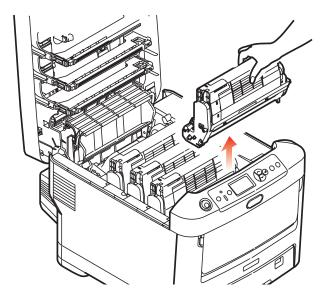
**4.** Put the assembly down gently onto a piece of paper to prevent toner from marking your furniture and to avoid damaging the green drum surface.
