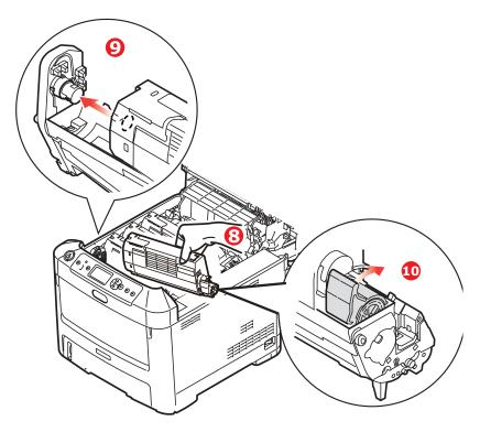
**10.** Pressing gently down on the cartridge to ensure that it is firmly seated, push the colored lever towards the rear of the printer. This will lock the cartridge into place and release toner into the image drum unit.
