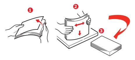
**3.** Load paper (letter headed paper face down and top edge towards the front of the printer), as shown.
