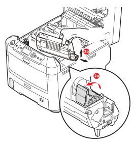
(b) Lift the right-hand end of the cartridge and then draw the cartridge to the right to release the left-hand end as shown, and withdraw the toner cartridge out of the printer.
