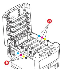
It will be necessary to remove the four image drums to gain access to the paper path.
