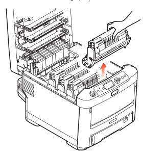
**5.** Put the assembly down gently onto a piece of paper to prevent toner from marking your furniture and to avoid damaging the green drum surface, and cover.
