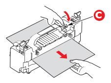
(e) Replace fuser unit into the machine and move locking levers (a) toward the rear of the machine.
