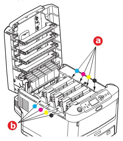
**3.** Lift each of the image drum units out of the printer and place them in a safe place away from direct sources of heat and light.
