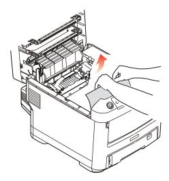
(b) To remove a sheet from the central area of the belt (2), carefully separate the sheet from the belt surface and withdraw the sheet.
