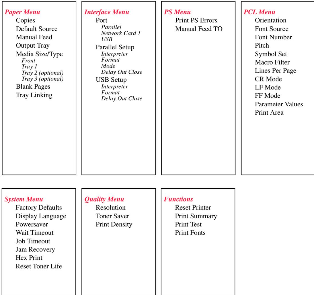
**Figure 1-3: Printer Menu Structure.**
