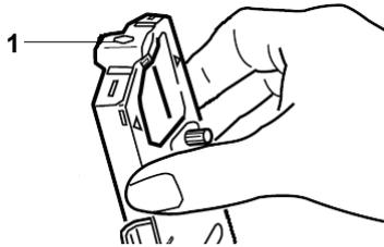
Remove the ribbon cartridge and check the ribbon shield.
