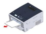
**)** Press the button (A) and open the output tray (a) completely.
