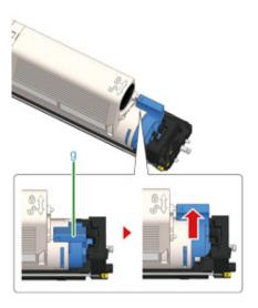
If you close the output tray without turning the blue lever when installing the toner cartridge into the image drum, it may cause a malfunction. Be sure to turn the blue lever until its top aligns on the lug in the back of the toner cartridge.
