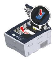
Tilt back the lock levers (c) on the both sides of the fuser unit toward you.
