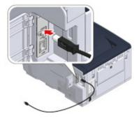
Pass the USB cable under the tab, and then close the interface cover.
