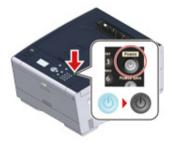
The "Shutting down. Please wait. Printer will turn off automatically." message is displayed on the display screen, and the power switch LED lamp flashes at approximately one-second intervals.
