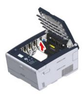
If paper jams in the fuser unit, press the jam release lever (b) on the fuser unit and slowly pull the jammed paper toward you.
