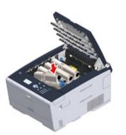
Hold the cartridge, pinch the tip of blue lever (b) of the toner cartridge, and turn forward until the tip aligns on the lug of the cartridge.
