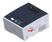
Siect the connector from the cover and connect with the wireless LAN module.
