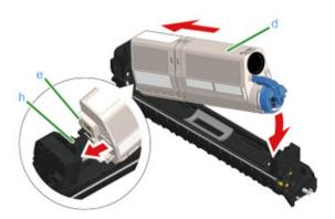
Hold the cartridge, pinch the tip of blue lever (g) of the toner cartridge, and turn forward until the tip aligns on the lug of the cartridge.
