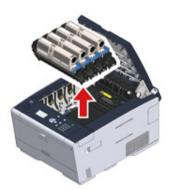
Cover the removed image drums with paper so that the image drums are not exposed to light.
