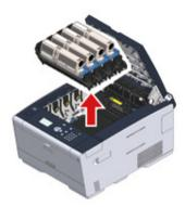
4 Cover the removed image drums with paper so that the image drums are not exposed to light.
