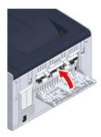
**)** Press the button (A) and open the output tray (a) completely.
