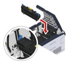
Tilt the lock levers on the both sides of the fuser unit.
