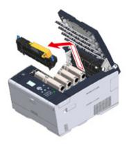
Push the blue lever on the fuser unit and remove the orange safety stopper and film.
