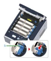
5 Lift the toner cartridge (c) from right side, and remove it from the machine.
