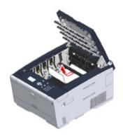
Hold the fuser unit handle and place the fuser unit into the machine.
