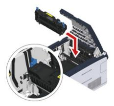
13 Tilt the lock levers on the both sides of the fuser unit.
