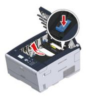
7 Tilt back the lock levers on the both sides of the fuser unit toward you.
