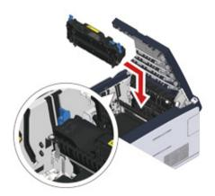
10 Tilt the lock levers (c) on the both sides of the fuser unit.
