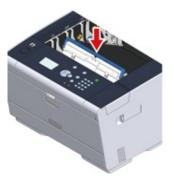
12 Turn the lock levers on the both sides of the belt unit forward.
