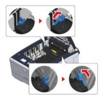
11 Replace the four image drums into the machine
