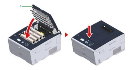
When the error message that the output tray is open does not disappear, make sure that the output tray is closed securely.
