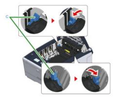
7 Hold the fuser unit handle and lift the fuser unit out of the machine.
