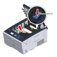
Tilt back the lock levers on the both sides of the fuser unit toward you.
