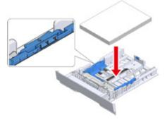
Secure the loaded paper with the paper guide.
