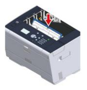
1 Turn the lock levers on the both sides of the belt unit forward.
