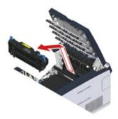
Turn the lock levers on the both sides of the belt unit toward you and remove the belt unit by holding the lock levers.
