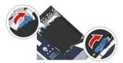
12 Hold the fuser unit handle and place the fuser unit into the machine.
