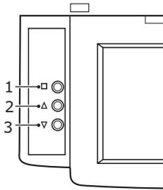
On the scanner unit control panel, press the Menu button (1) to display the OSD then press the Up-arrow (2) or Down-arrow (3) buttons to reach the required function. Press the Menu button, use the Up-arrow and Down-arrow buttons to locate the required option then press the Menu button to set the option and return to the OSD main menu.
