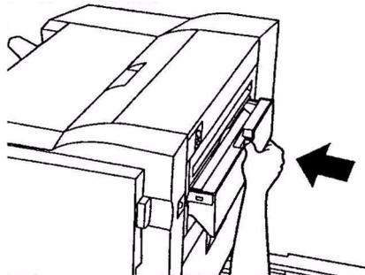
5. Check that the punch chip box has been replaced correctly then move the Finisher back into position, being careful not to trap your fingers.
