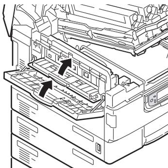
10. Return the image drum basket (9) into position and check it is locked.
