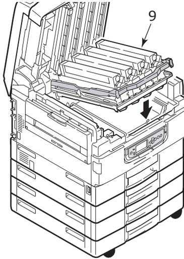
11. Close the printer unit top cover and ensure it is latched, then lower the scanner unit.
