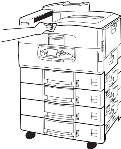
3. Use a soft dry cloth to dry the printer unit surface.
