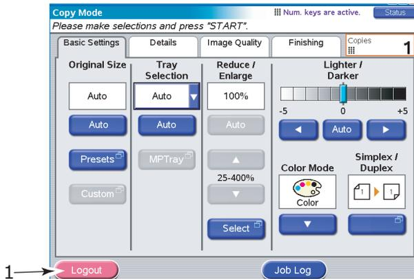
1. When you have finished using the scanner unit, press the Logout button (1) to return to the access control screen.
