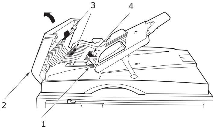
3. Wipe the feed rollers (3) by moving the swab from side to side.
