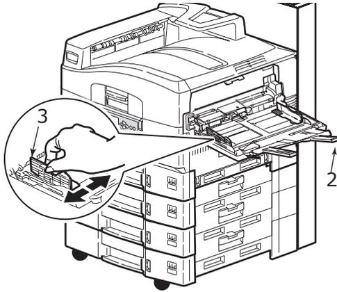
3. Adjust the paper guides (3) to the size of the paper being used.
