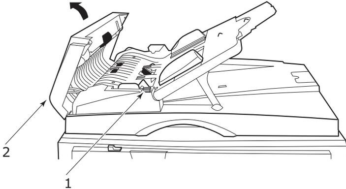
2. Press both arms of the ADF snap-in pad module inward with your fingers and pull out the ADF snap-in pad module.
