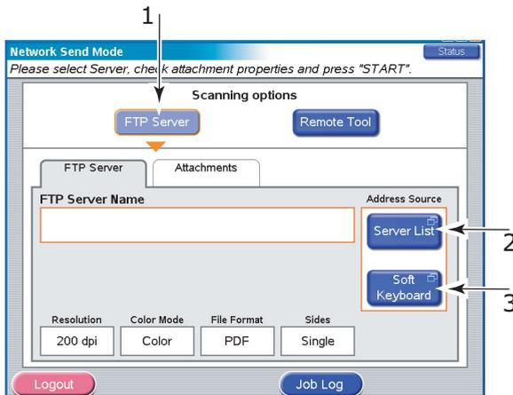
2. Press the FTP Server button (1) (set by default) and enter an FTP server name via one of the following buttons:
