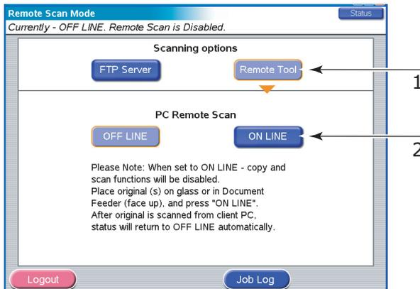
2. Press the Remote Tool button (1) to enter PC Remote Scan mode in the Off Line status.
