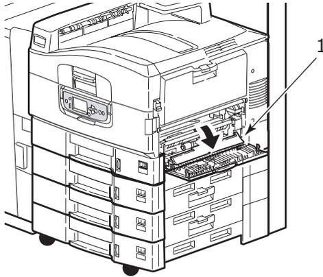
3. Remove Tray 1 completely from the printer unit.
