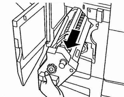
5. Turn the knob in the direction indicated to move the stapler to the front.
