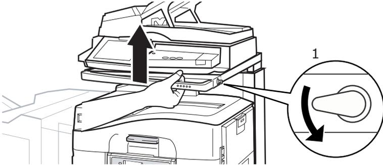
2. To open the top cover, squeeze the top cover handle (1) to release the catch and raise the cover.
