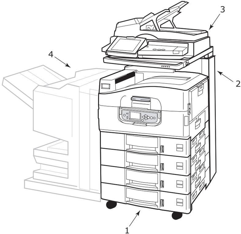
1. Printer unit (with high capacity feeder (HCF))
