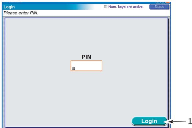
2. Press the Login button (1) and the default Copy Mode screen appears, the scanner unit now being available to use.
