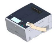
**3** Dry the surface of the machine with a dry soft cloth.
