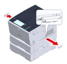
5 Lift up the machine to remove the additional tray unit.
