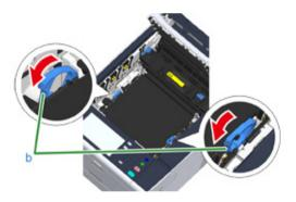
6 Remove the belt unit by holding the lock lever (b).
