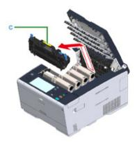
**5** Push the blue lever on the new fuser unit and remove the orange safety stopper.
