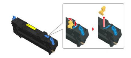
6 Hold the handle of a new fuser unit, align the fuser unit to the grooves behind the toner cartridges, place the fuser unit into the machine.
