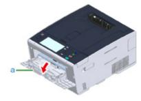
2 Slightly lifting the MP tray (a), press the right arm (b) inward, then unlock the tab (c).
