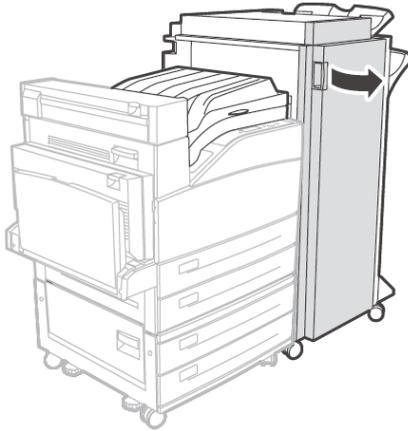
**17.** Remove the internal tags and shipping brackets.
