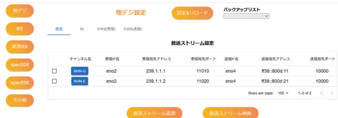
Figure 2. Example of IP Broadcast Server's Configuration Display
