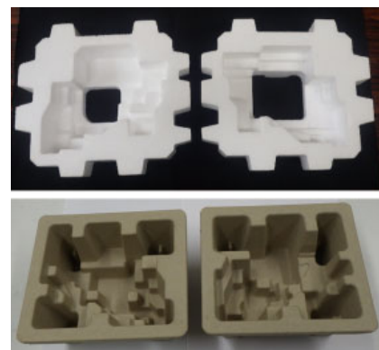
Photo 6. Cushioning Materials Top: EPS, Bottom: Molded Pulp
