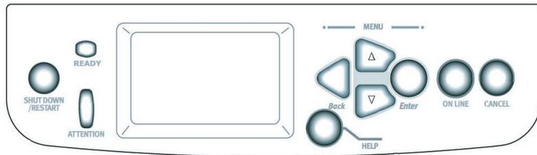
Use the Control Panel to view status information, print special pages, and set up printing. While most elements in the Control Panel display have counterparts in Command WorkStation, you can view current functions on the Control Panel even when Command WorkStation is not connected to the server or is not running.
