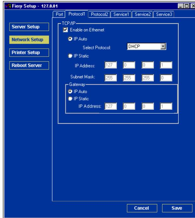
You can change TCP/IP, AppleTalk and IPX/SPX protocol settings for the Fiery. Change these settings on the Protocol1 and Protocol2 tabs.
