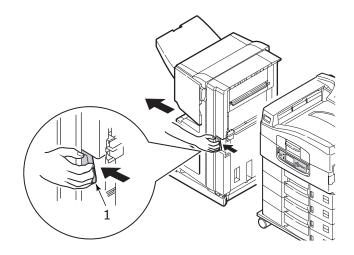
**2.** Operate the duplex cover release button (2) and open the cover.
