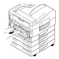
**4.** Operate the levers (3) and pull out the duplex unit.
