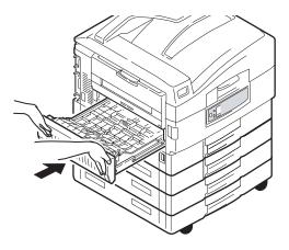
**10.** If you detached a Finisher unit to gain access to the duplex unit, replace the Finisher unit.
