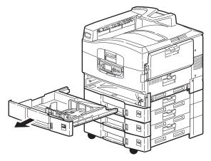
**4.** Gaining access through the gap left by Tray 1, wipe the 3 paper feed rollers (2) with a soft cloth lightly moistened with water.
