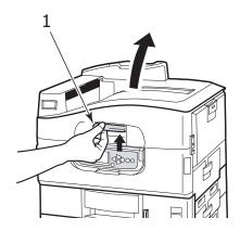
To close the top cover, push gently (1) until the cover stops midway and then push harder (2) to close the cover completely. Ensure that the cover is securely closed.
