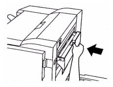
**5.** Check that the punch chip box has been refitted correctly then move the Finisher back into position, being careful not to trap your fingers.
