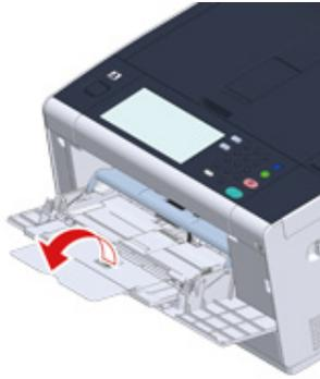
4 Adjust the manual feeding paper guide to the width of paper to be loaded.
