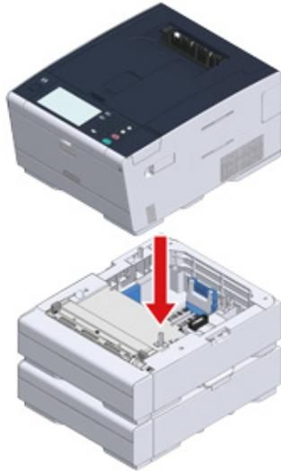
**4** Screw the machine and additional tray unit with the lock pieces.
