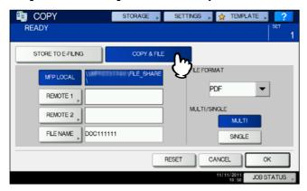
**4** Press the necessary buttons for entering information about the data to be stored. Then press [OK].
