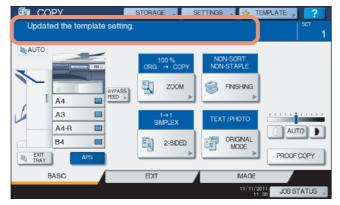
**9** Select other copy modes as required, and then press the [START] button on the control panel.
