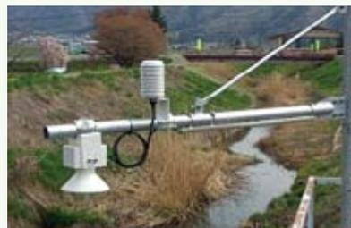
Water level indicator for measuring water at an observation point
