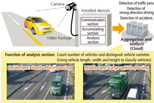
Traffic flow analysis system using video sensing
