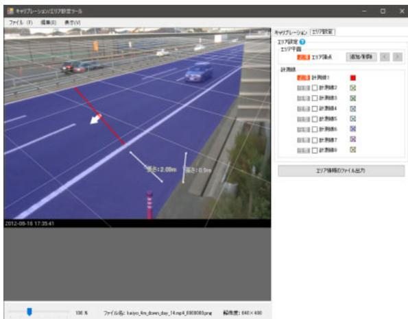
**Photo 3. Area/Measurement Line Setup Screen**
