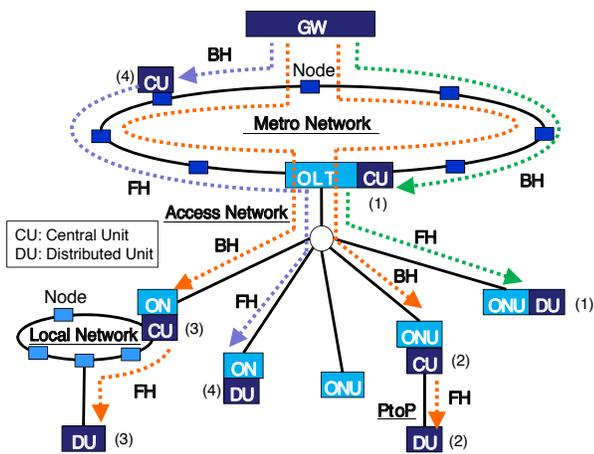
**Figure 2. Line Allocation in a PON System**
