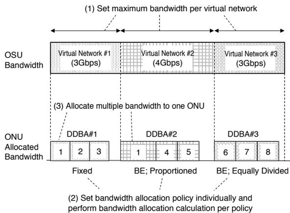
**Figure 7. Example Configuration for Domain DBA**
