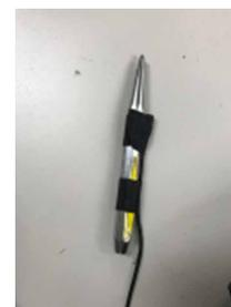
**Figure 6. Metal Rod and Microphone used in Crack Test**
