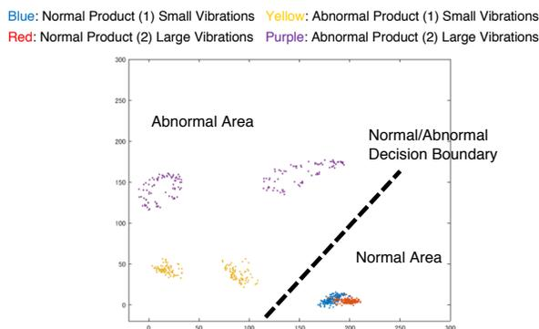
**Figure 4. Decision based on OKI's Vibration Analysis Algorithm**
