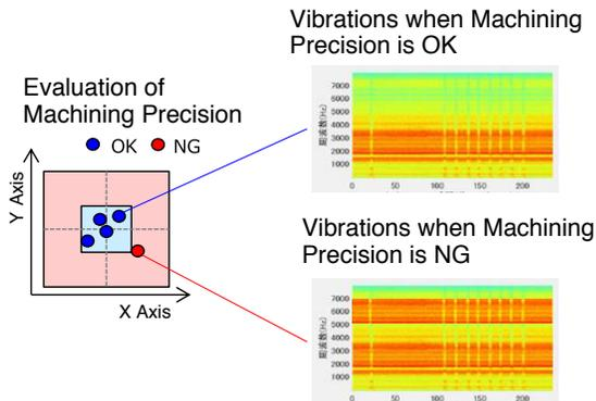
**Figure 8. Correlation between Machining Precision and Vibration**
