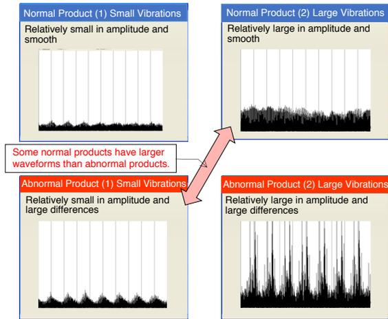
**Figure 3. Vibration Data of Normal/Abnormal Motors**
