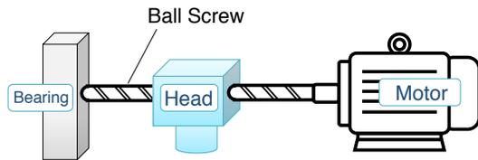
**Figure 7. General Ball Screw Mechanism**
