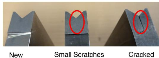
**Figure 5. Crack in Press Mold**
