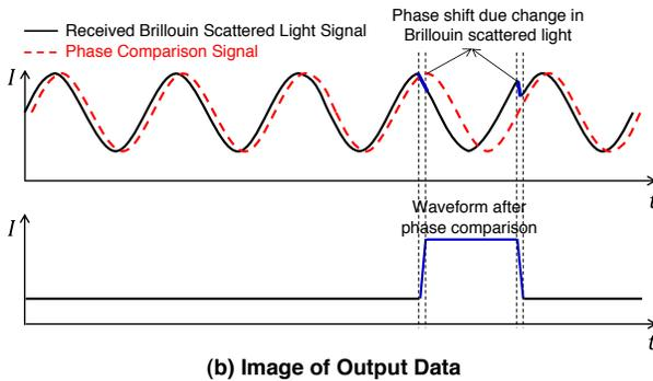
**Figure 2. SDH-BOTDR Configuration and Image of Output Data**
