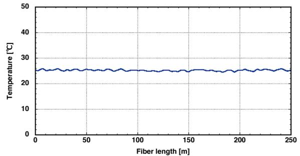
(b) Result of Distributed Temperature Measurement in Factory (Example)
