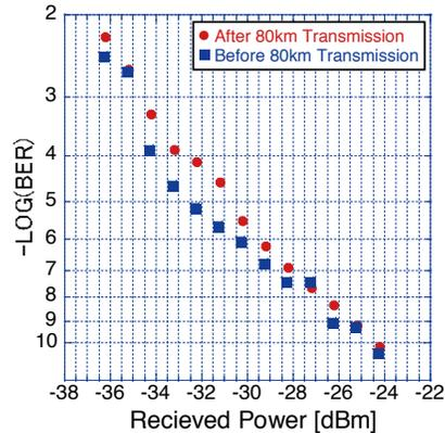
Figure 6. Symbol Error Rate of 25Gbaud-QPSK
