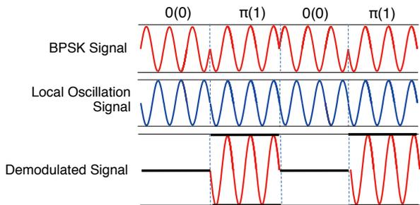
Figure 1. Detection Example of BPSK
