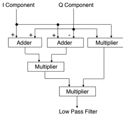
Figure 5. Calculation Required for Phase Error Extraction in QPSK
