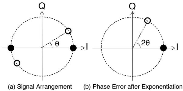
Figure 3. BPSK Signal Arrangement
