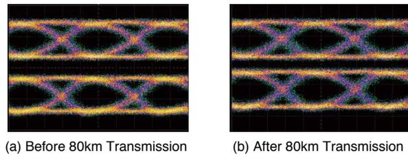
Figure 7. Eye Pattern of Demodulated Waveform
