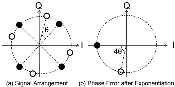
Figure 4. QPSK Signal Arrangement
