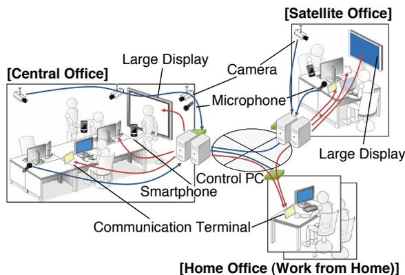
Figure 4. Ultra-Realistic Telework System
