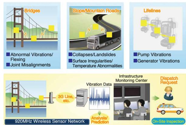
Figure 1. Social Infrastructure Monitoring System Utilizing 920MHz Wireless Sensor Network
