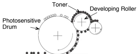
Figure 9. Single-Component Contact Development System
