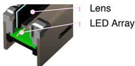
Figure 8. LED Print Head Components
