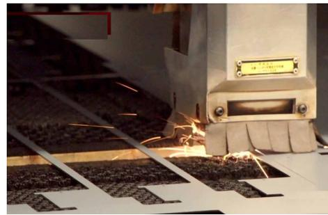
Photo 4. Contour Cutting using a Laser
