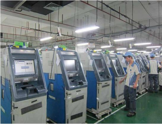
Photo 8. Final Inspection of ATM-Recycler G7
