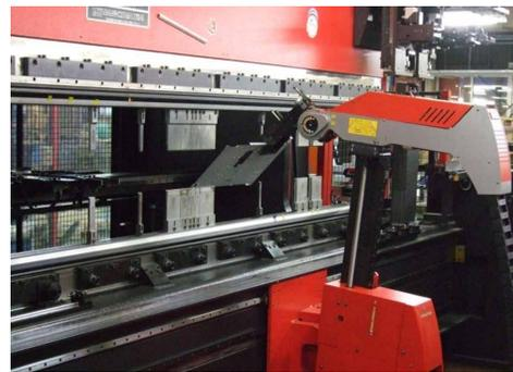
Photo 5. Automation of Bending Process
