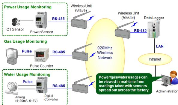
Figure 5. Conversion of Various Sensor Interfaces to Wireless
