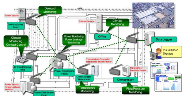
**Figure 4. Placement of Various Sensors at a Factory**
