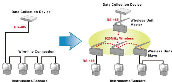
Figure 2. RS-485 Connections Replaced with Transparent Model
