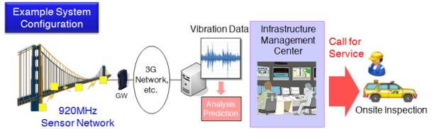
Figure 6. Structure Monitoring System using Wireless Sensors
