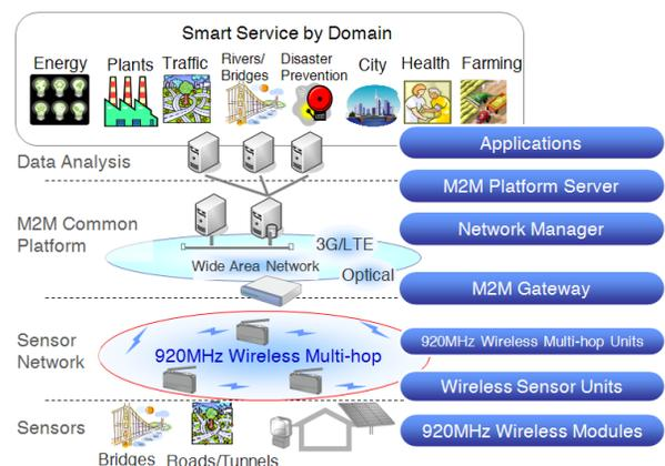
Figure 1. OKI's M2M Solution Configuration
