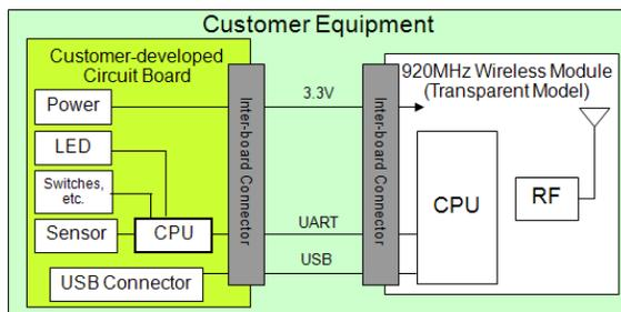
**Figure 3. Configuration using Transparent Model**
