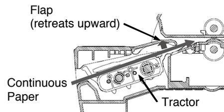
Figure 8-2. Tractor and Flap (Continuous Paper)
