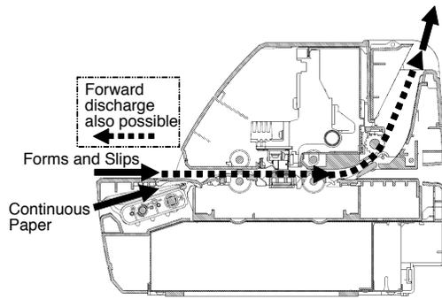
Figure 6-2. Upward Discharge Passage
