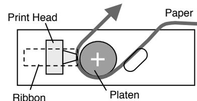
Figure 2. Basic Design of Round Type Printer
