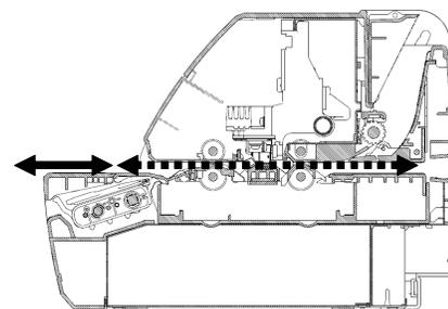
**Figure 6-1. Horizontal Discharge Passage**
