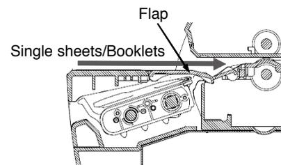
Figure 8-1. Tractor and Flap (Single Sheet Paper)
