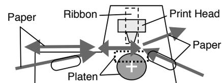
Figure 3. Basic Design of Flatbed Type Printer
