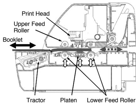
Figure 7. Completely Horizontal Transport System
