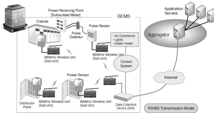
Figure 8: Configuration Example: BEMS
