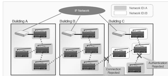
Figure 1. Independent Network Configuration
