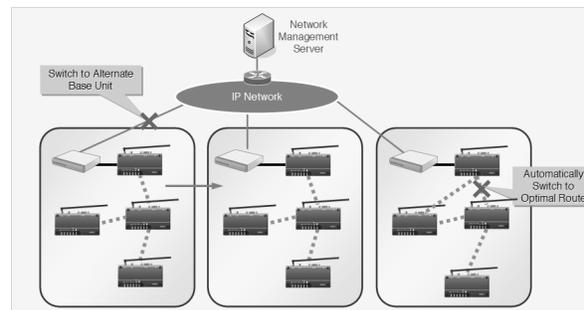
Figure 2. Dynamic Routing Function
