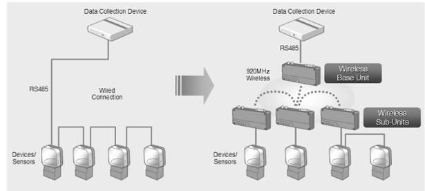
Figure 4. RS485 Transmission Model
