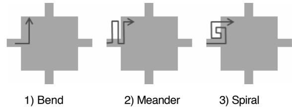
**Figure 4. Bridge Line Design Methods**
