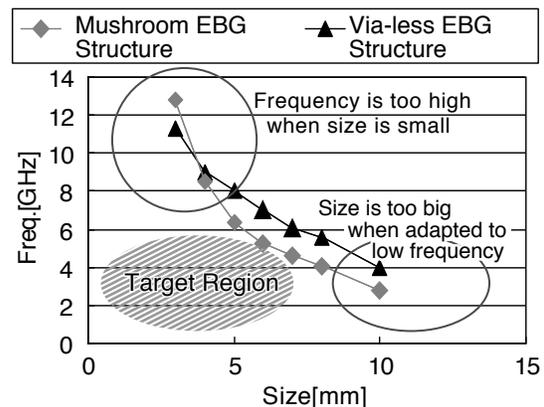
Figure 2. Stopband and Unit Cell Size
