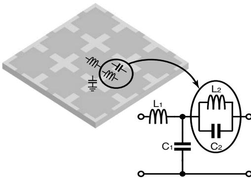
**Figure 3. Equivalent Circuit of Via-less EBG Structure**
